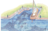
Sheltered Embayment: Inner Harbour Quay Restoration - Inner harbour quay treatments using structural habitat such as anchored logs, floating docks, and rock gravel shoals and reefs
